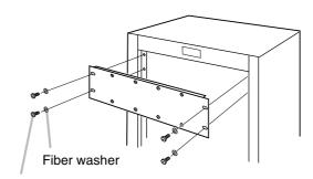
Binding head self tapping screw (5 x 12)
